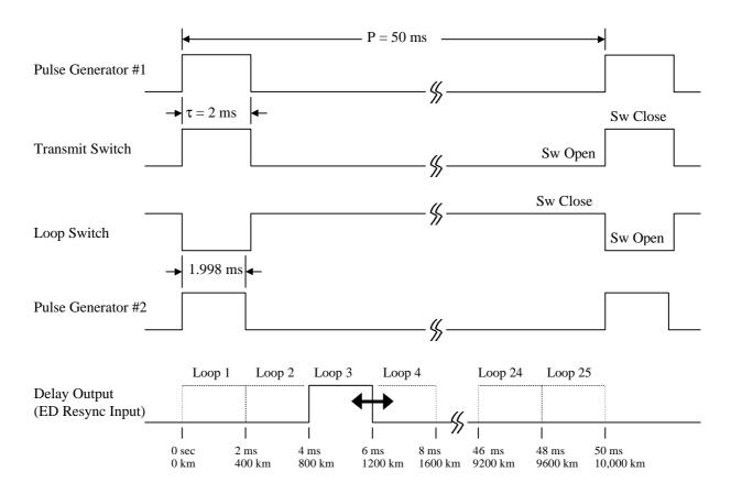
Figure 2: Example Circulating Loop Timing Diagram
